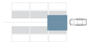
In structures without a turntable, vehicles enter and exit parallel to the rack structure.
