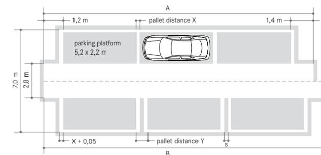
The distance between the parking platforms is depending on the height of the parking system: x without wallplates / y including wallplates of 30 cm
